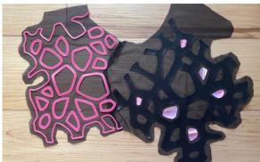
Figure 3. Muslin prototype of SMA wire corded petals.
